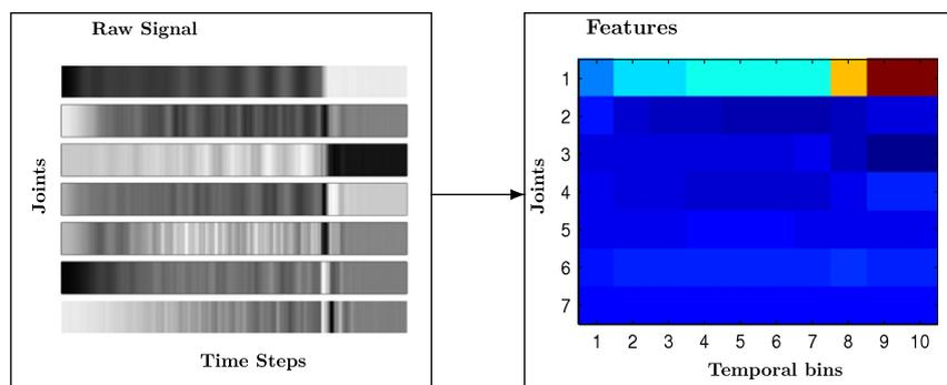
**Fig. 5.** Illustration of the proprioceptive feature extraction routine. The input signal is sampled during the execution of a behavior at 500 Hz and consists of the raw torque values for each of the robot's seven joints. Features are extracted by discretizing time (horizontal axis) into 10 temporal bins, resulting in a  $7 \times 10 = 70$  dimensional feature vector.
