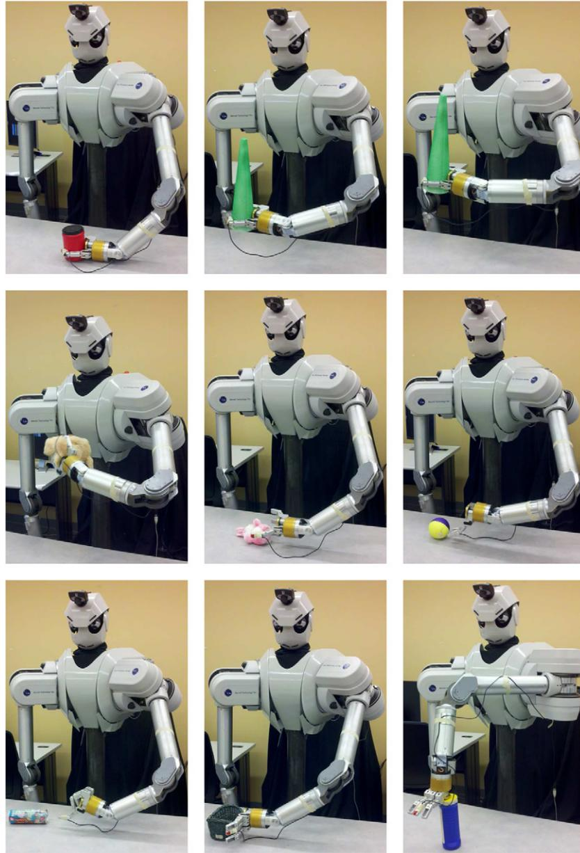
**Fig. 4.** The exploratory behaviors that the robot performed on all objects shown in Fig. 2. From top to bottom and from left to right: (1) grasp, (2) lift, (3) hold, (4) shake, (5) drop, (6) tap, (7) poke, (8) push, and (9) press. The look behavior is described in Fig. 3.
