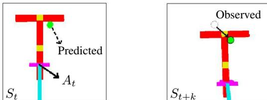
Fig. 1. A sample trial with the T-stick tool. At the start of the trial (left), the robot makes a prediction regarding the outcome of its tool action,  $A_t$ , based on the current sensory input,  $S_t$ . Once movement of the puck is detected, the robot is able to verify its prediction by comparing it with the observed outcome (right).
