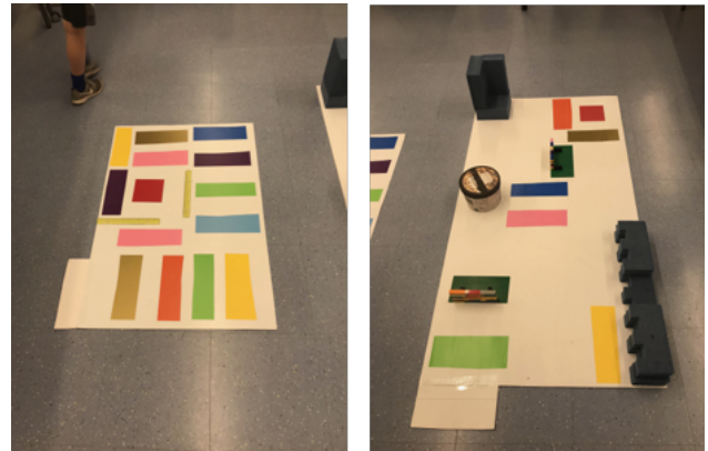
Figure 4: Two mats used in our pilot study. In the first (left), some colors are difficult to detect by the robot's sensor; In the second mat (right) some surfaces confuse the robot's distance sensor. For both mazes, the robot was tasked to drive around on the mat but never leave it (using the obstacles or color strips to stay on the mat).
