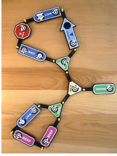
Figure 4: This program features two concurrent tasks. The left branch causes the robot to emit two beeps every three seconds. The right branch starts a motor, waits for a touch sensor to be released, stops the motor, and then repeats.
