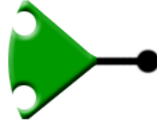
Figure 4.5: The merge statement combines two branches of code split by an if-statement.
