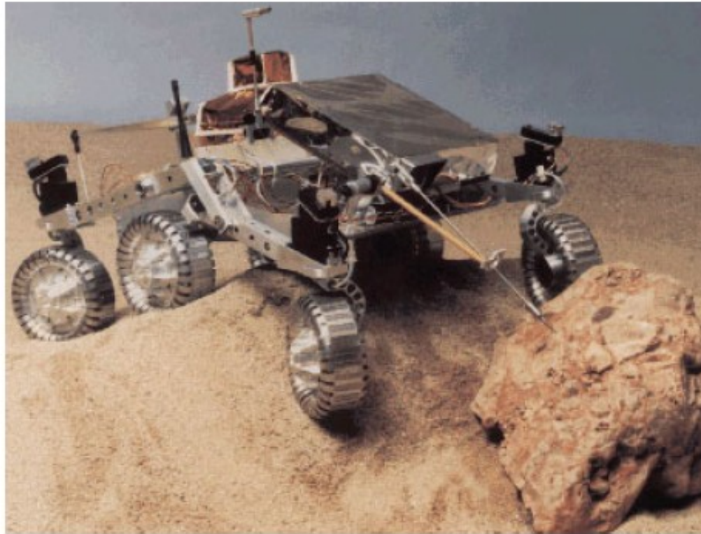
Figure 1.7 Sojourner Mars rover. (Photograph courtesy of the National Aeronautics and Space Administration.)
