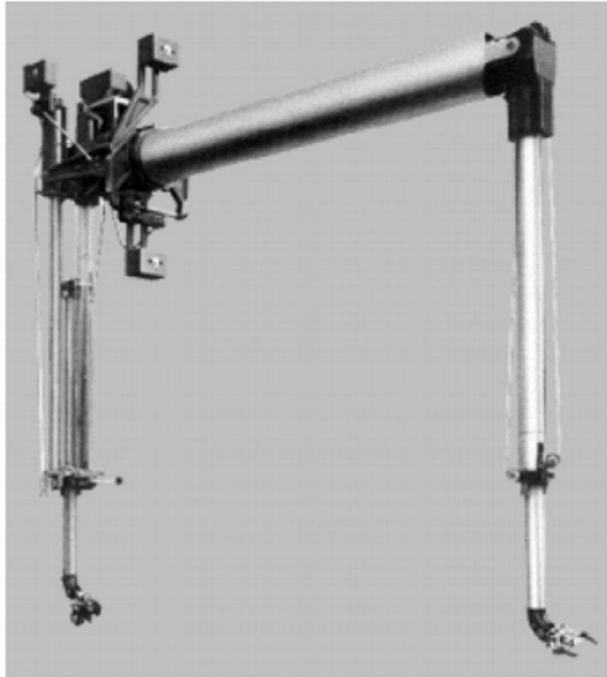
Figure 1.2 A Model 8 Telemanipulator. The upper portion of the device is placed in the ceiling, and the portion on the right extends into the hot cell. (Photograph courtesy Central Research Laboratories.)
