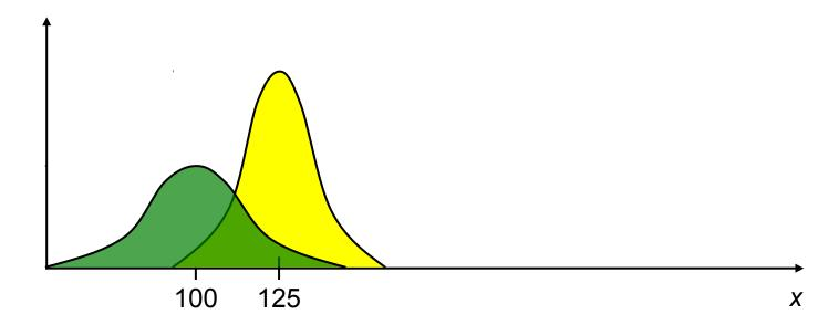
$$\mu = \left[ \frac{\sigma_{z_2}^2}{\sigma_{z_1}^2 + \sigma_{z_2}^2} \right] z_1 + \left[ \frac{\sigma_{z_1}^2}{\sigma_{z_1}^2 + \sigma_{z_2}^2} \right] z_2$$
