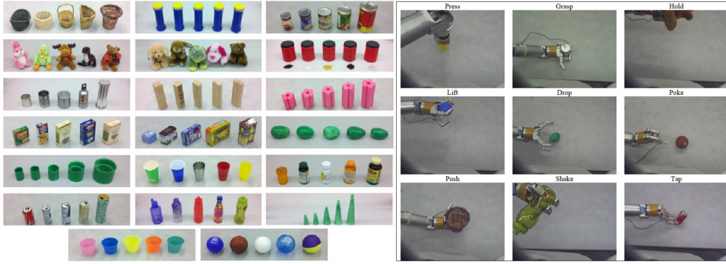
Figure 7.3: Left: 100 objects, grouped in 20 object categories. Right: The interactive behaviors that the robot performed on the objects. From top to bottom and from left to right: (1) press , (2) grasp , (3) hold , (4) lift , (5) drop , (6) poke , (7) push , (8) shake and (9) tap .
