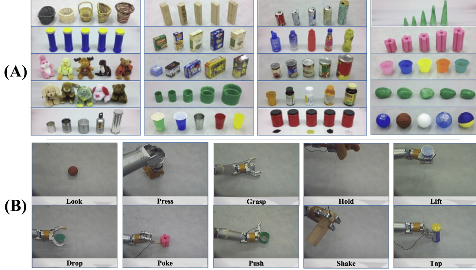
Figure 10.2: (A) 100 objects, grouped in 20 object categories. (B) The interactive behaviors that the robot performed on the objects.
