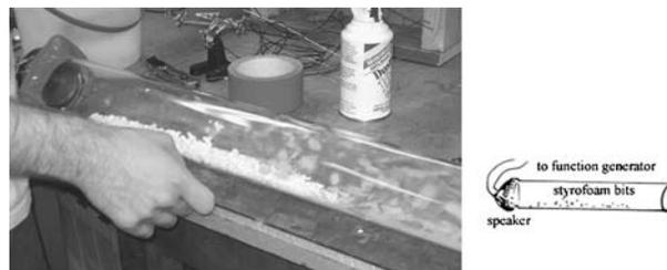
Figure 4. Left: Speaker taped to clear tube filled with Styrofoam bits. Right: Diagram.
