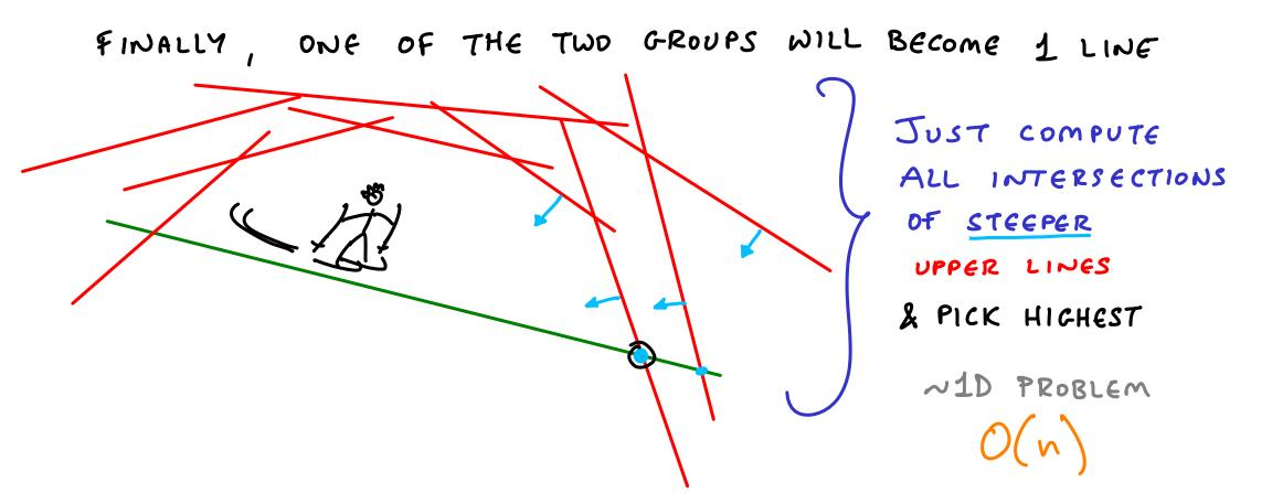
0) ROTATE COORDINATE SYSTEM 1) PAIR LINES upper w/ upper j lower w/ lower 2) COMPUTE MEDIAN OF 1/2 INTERSECTION POINTS 3) PERFORM VERTICAL TEST & FIND SIDE CONTAINING MIN 4) FOR PAIRS ON WRONG SIDE, DISCARD 1 LINE 5) IF STILL >1 LINE IN EACH SET, REPEAT FROM (1) ON 3/4 of the lines 6) EASY SOLUTION WHEN ONLY 1 LINE IN A SET.
