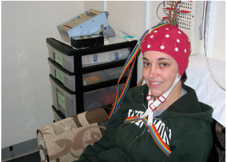
Figure 1: Unlike some BCI systems that require inserting devices directly into the brain, EEG electrode caps are worn externally.
